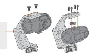
The FAST™ FTC OMNI mount uses a force-to-overcome mechanism. Grasp the magnifier body and pivot assembly down to the stowed position. Repeat in reverse to bring the magnifier back into the active position.
