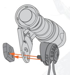
Install Remora™ into MARK™ as shown. Note Remora is compatible with all versions of MARK.
