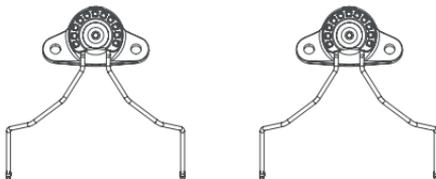
Two (2) ARC Rail Adapter Plates (Note: Not used on Team Wendy® EXFIL® rails.)
