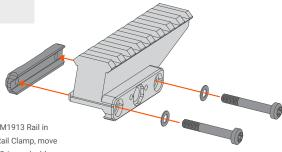
Place the FAST™ Absolute Riser on the M1913 Rail in desired location. If using the included Rail Clamp, move to step 2. If using the optional FAST™ QD Lever (sold separately), jump to step 3.
