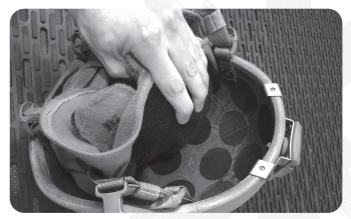
Remove CWL™ by grasping entire liner / pad assembly and slowly pulling it out of the shell. Take care to not tear fabric or stitching. Once removed, pull pads out of CWL™ and replace them in helmet.
