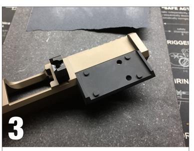
Clean the adapter plate and test fit after every 4-5 passes on each dovetail surface. The plate should fit snug and offer slight resistance while inserting into the slide dovetail.
