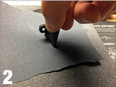
Keeping the sandpaper flat, carefully rest the adapter on its dovetail face and rub along the sandpaper using light pressure, careful to keep the dovetail surface flat and at the correct angle.
