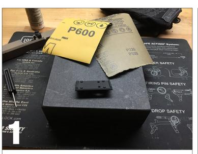
If adapter plate requires fitting, just grab a piece of fine grit sandpaper (320-600) and a flat surface to work on.
